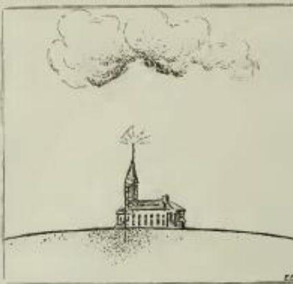
Fig. 4. Testa Explains the Fallacy of the Franklin Pointed Lightning Rod, Here Illustrated, and Shows that Usually Such a Rod Could Not Draw Off the Electricity in a Single Cloud in Many Years. The Density of the Dots Indicates the Intensity of the Charges.
